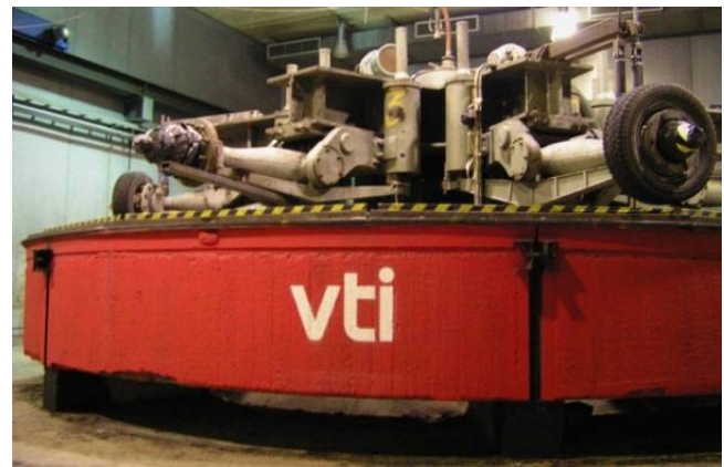
Fig. 1: The VTI's Circular Road Simulator, photo after VTI Image Database, 2016
